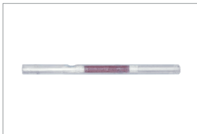
Illustration of amalgam trap. Increase sensitivity by a factor of 100 and reduces spectral noise.
