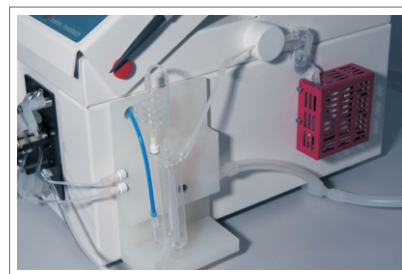
Illustration of the mercurio-CV „wet chemistry system“, which is easily accessible outside the device.
