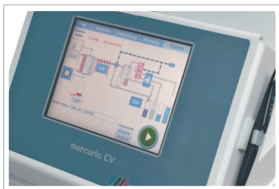
Illustration of the computer terminal with touch input, high-resolution color monitor and the easyCONTROL operating and evaluation program.
