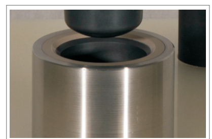
Milling-set protected by stainless steel jacket
